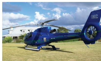
The spacious, air-conditioned cabin with raised rear seating offers breathtaking wraparound Views, while the unique fenestron tail rotor minimizes noise both inside and out.
